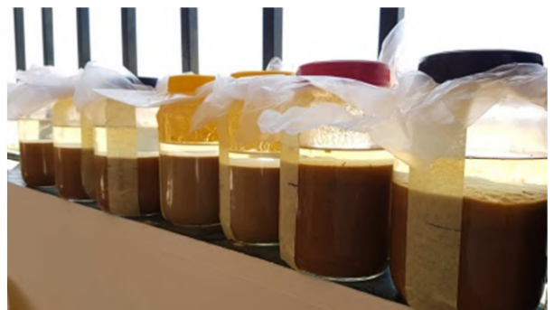
Figure 4. Jar tests at MSA CoE, Egypt.
