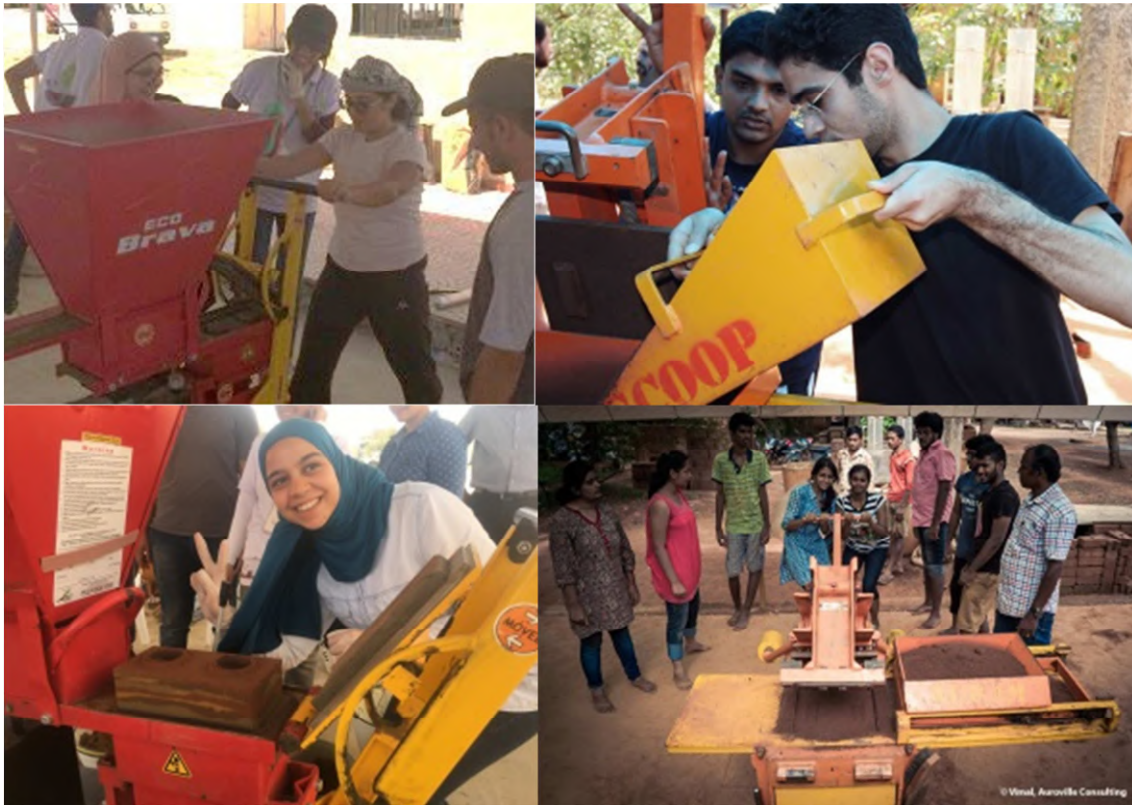
Figure 9. Producing CSEB using Eco Brava machine (left) and Auram 3000 machine (right).
