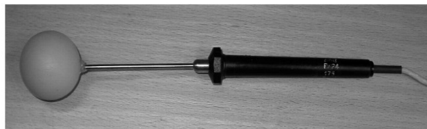
Fig. 3 The 38 mm flat grey globe thermometer (Thorsson et al., 2007a)
