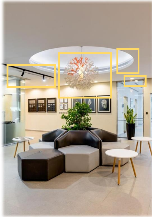
Figure (18): Using many types of artificial lighting: Indirect light, spotlights, as well as pendant and track light
