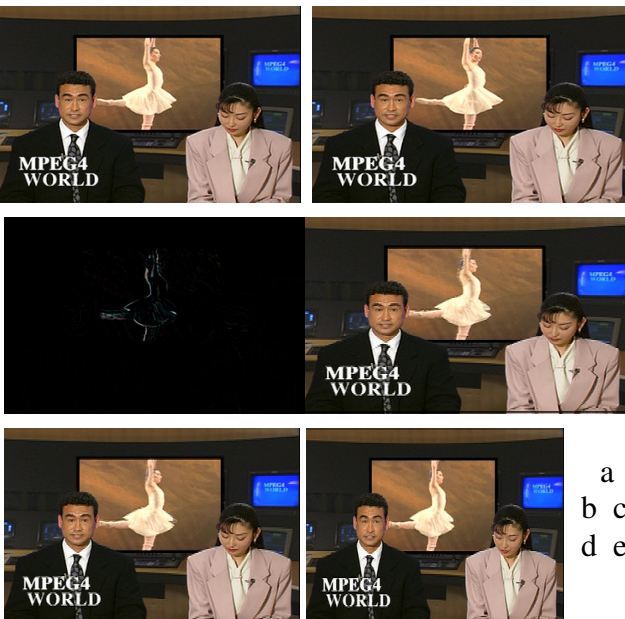
Figure 4: Motion Detectors. a. 4 th and 5 th Progressive Frames, b. Difference of 1 st and 2 nd Progressive Frames, c. Interpolation Using 3-Field Motion Detector, d. Interpolation Using 4-Field Motion Detector, and e. Interpolation Using 5-Field Motion Detector.
