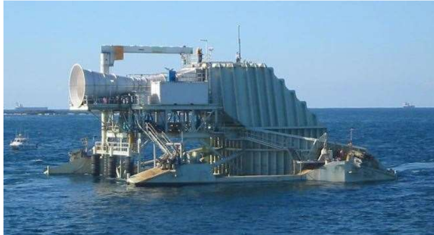
Figure 4.6 Oscillating Water Column: OceanLinx [42].
