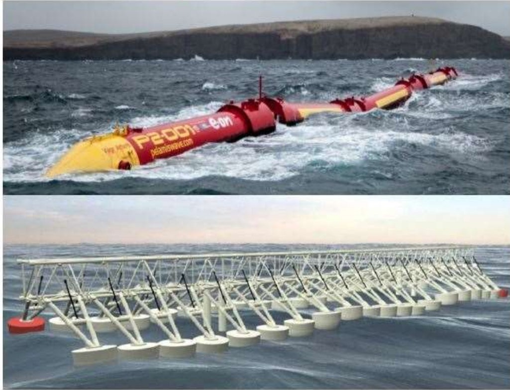
Figure 4.4 Attenuator: Pelamis (top) [46] and Wave Star (bottom) [47].
