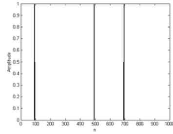
Fig. 7 (a) Signal after (CA-CFAR)
