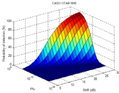
Fig. 2 (b) SO-CFAR processor
