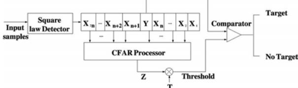
Figure 1. (a) Block diagram of typical CFAR processor
