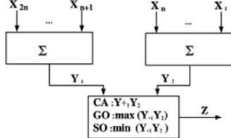
Figure 1. (b) Mean-level CFAR processors.
