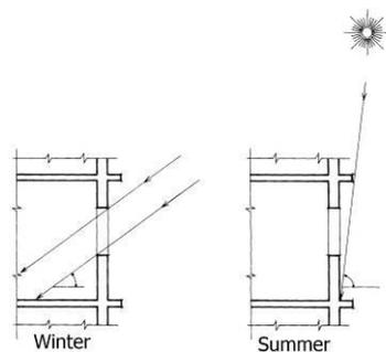
Figure 16: Small overhang shading device on the southern façade (Fathy, 1986)
