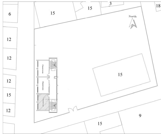
Figure 1: Case study 1 layout Notes: a) classroom under investigation is hatched b) Numbers on surrounding buildings are their height in meters
