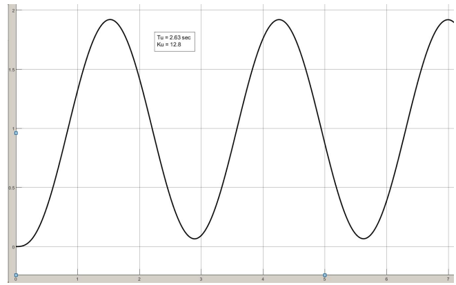
Fig. 6: The sinusoidal ZN cruise system response.
